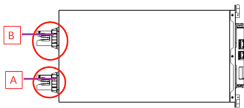
Figure 1-4 Schematic diagram of the location of the NO HANDLING points A and B
